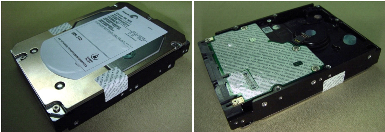
Figure 7. Example of FIPS tamper evidence labels.
