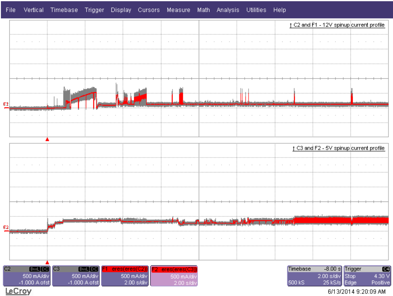
Figure 2. Current profiles for 1TB models
