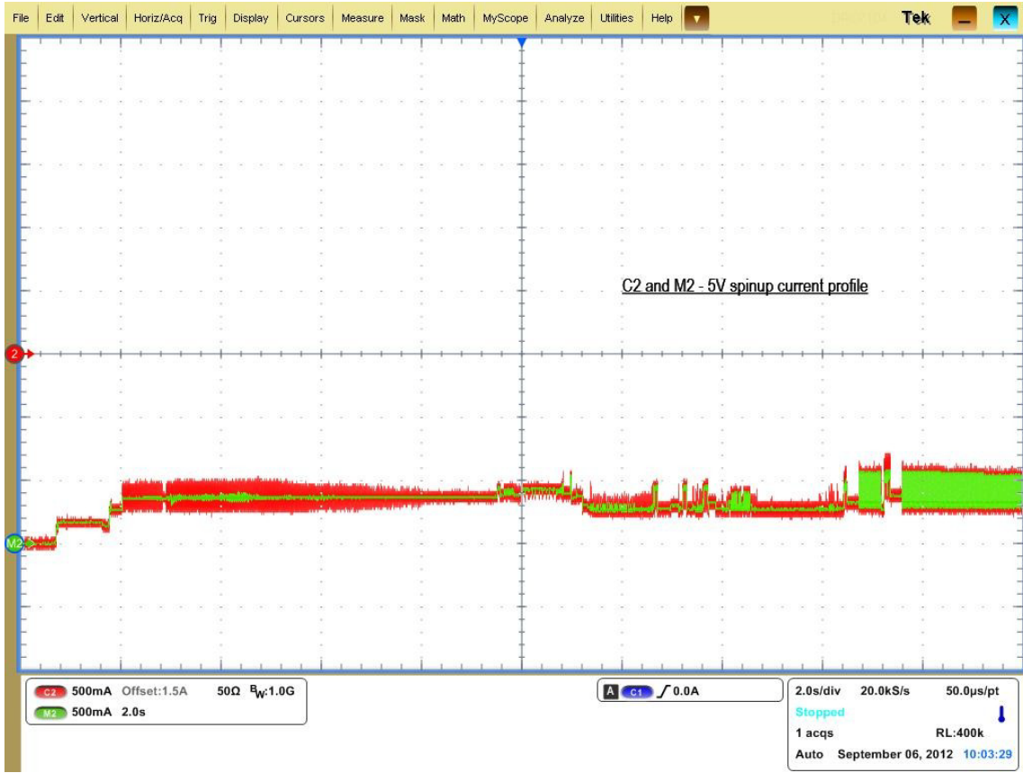
Figure 1. 4TB Typical 5V startup and operation current profile
