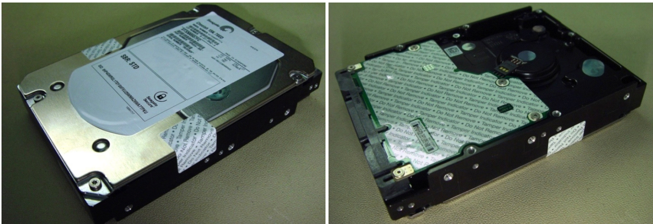
Figure 14. Example of FIPS tamper evidence labels.
