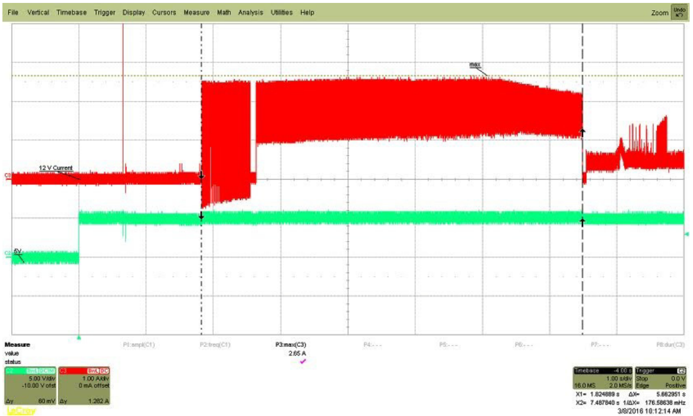
Figure 2. 4TB Typical 5V and 12V startup and operation current profile
