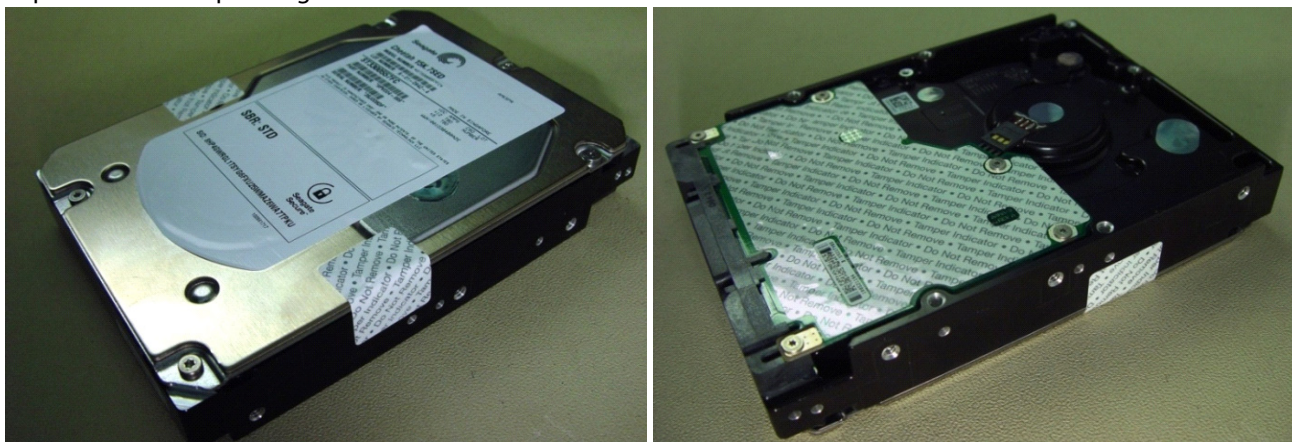
Figure 4. Example of FIPS tamper evidence labels.
