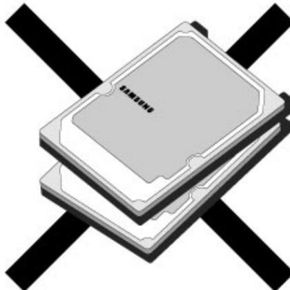
Fig. 9-3: HDD handling guide -Do Not Stack!
