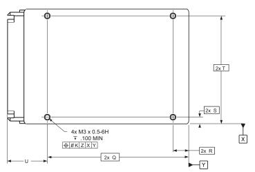
Figure 12. Mounting configuration dimensions
