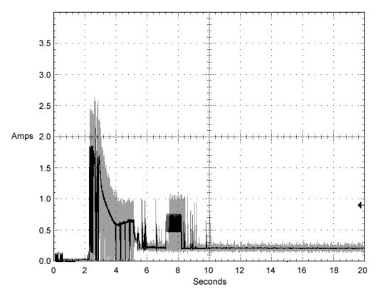
Figure 2. Typical ST973401 drive +12 V current profile
