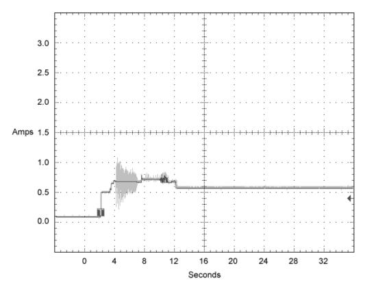
Figure 3. Typical ST973401 drive +5 V current profile
