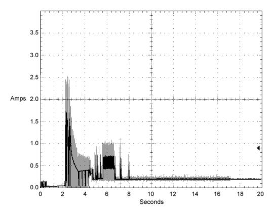
Figure 4. Typical ST936701 drive +12 V current profile
