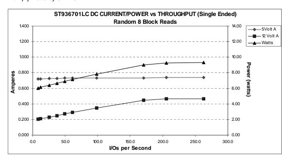
Figure 8. ST936701 DC current and power vs. input/output operations per second (SE)
