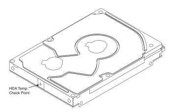
Figure 10. Location of the HDA temperature check point
