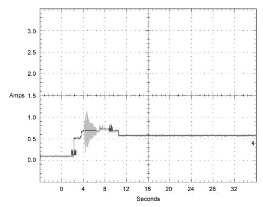
Figure 5. Typical ST936701 drive +5 V current profile
