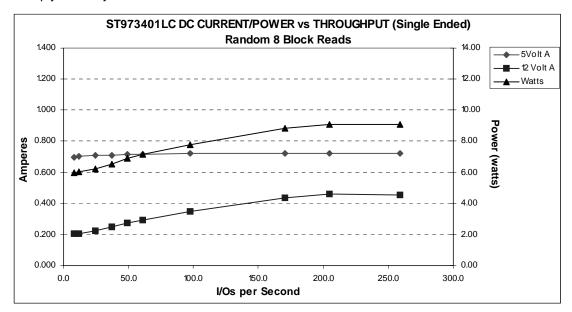
Figure 6. ST973401 DC current and power vs. input/output operations per second (SE)
