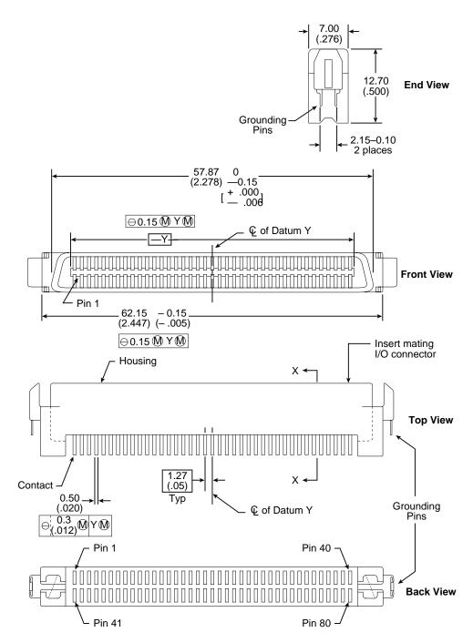
Figure 15. Nonshielded 80-pin SCSI "SCA-2" connector
