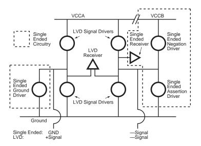
Figure 16. Typical SE-LVD alternative transmitter receiver circuits
