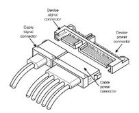
The Serial ATA interface cable consists of four conductors in two differential pairs, plus three ground connections. The cable size may be 30 to 26 AWG with a maximum length of one meter (39.37 in).
