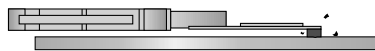
Head slaps the disc, causing damage and leaving particles on the disc.
