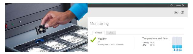
The 8-bay rackmount NAS includes redundant power supplies to keep your business up running. If you ever need to change a power supply, it's as simple as depressing a tab and sliding it out — no tools required.
