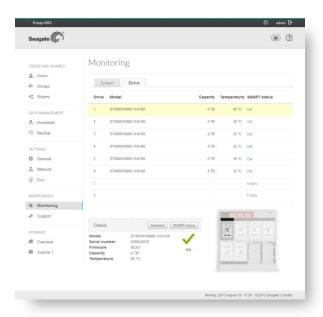
In the same menu under the "Drive" tab, you will see the status of each drive installed in the system. When you click on a drive number or other info in the list, an image below will highlight where the drive is installed in the system.
