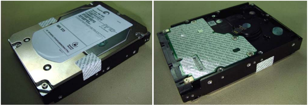
Figure 16. Example of FIPS tamper evidence labels.
