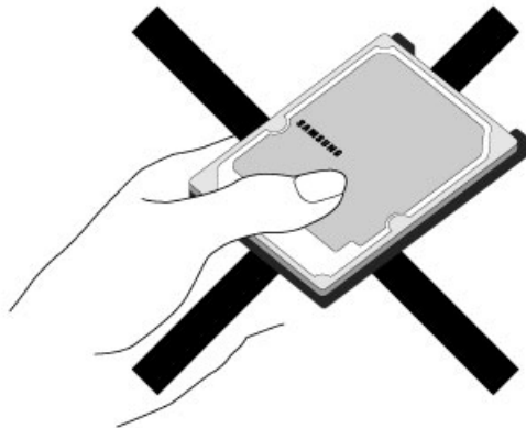
Fig. 9-2: HDD handling guide -Do not Touch Cover and PCB!
