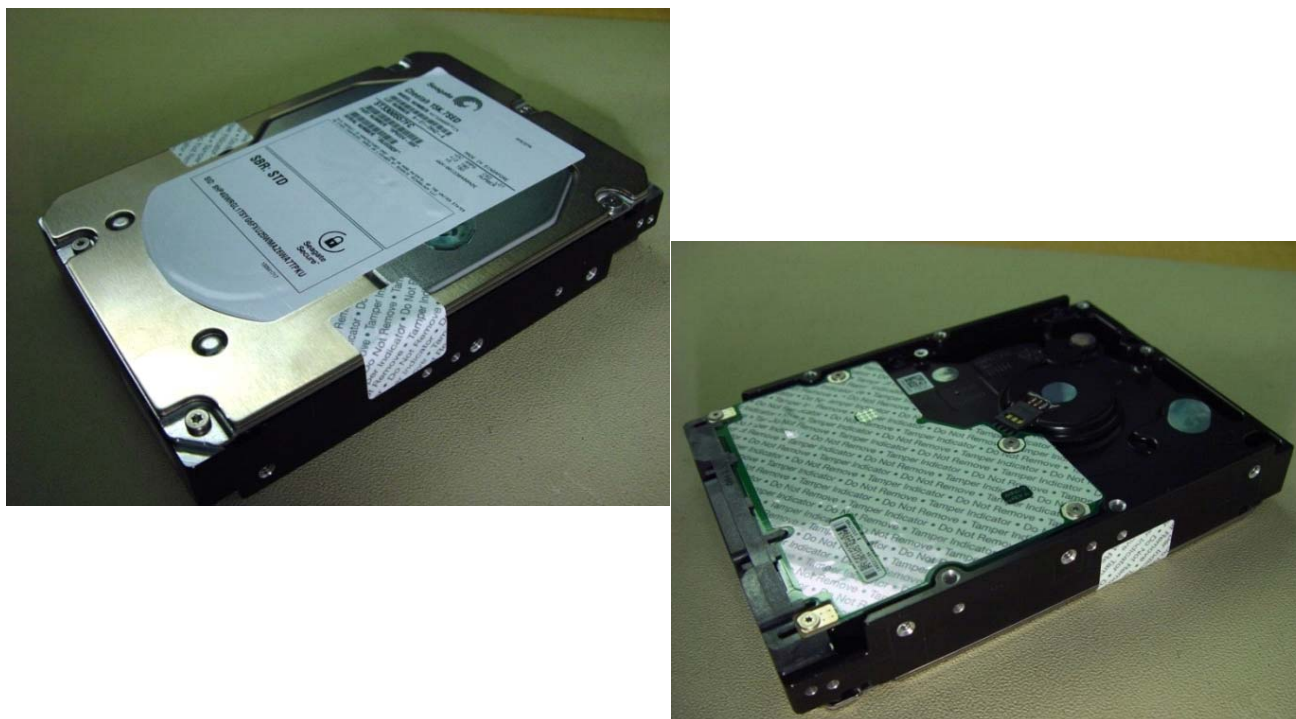
Figure 10. Example of FIPS tamper evidence labels.
