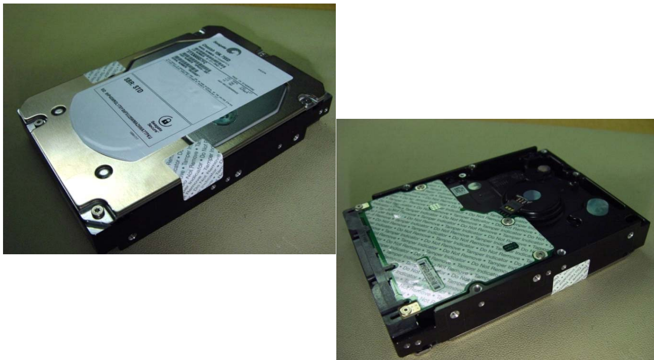
Figure 10. Example of FIPS tamper evidence labels.
