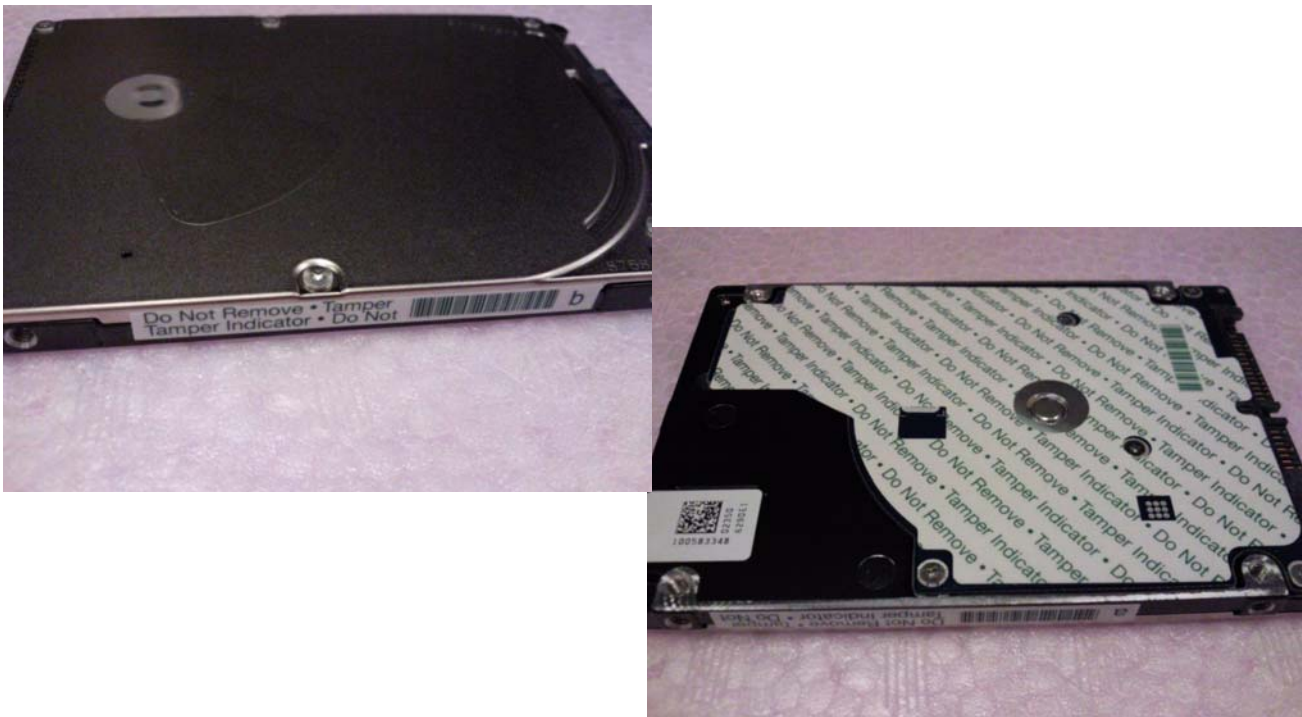
Figure 6. Example of FIPS tamper evidence labels.
