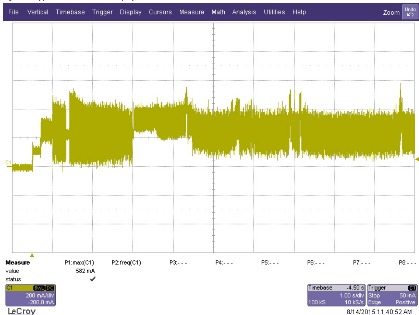
Figure 2 Typical Current Profiles (5V)
