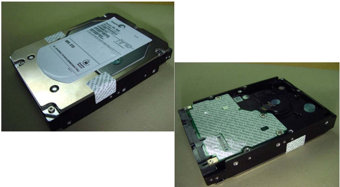
Figure 10. Example of FIPS tamper evidence labels. Note. Does not represent actual drive.
