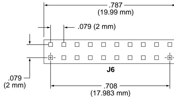
Figure 15. J6 connector dimensions
