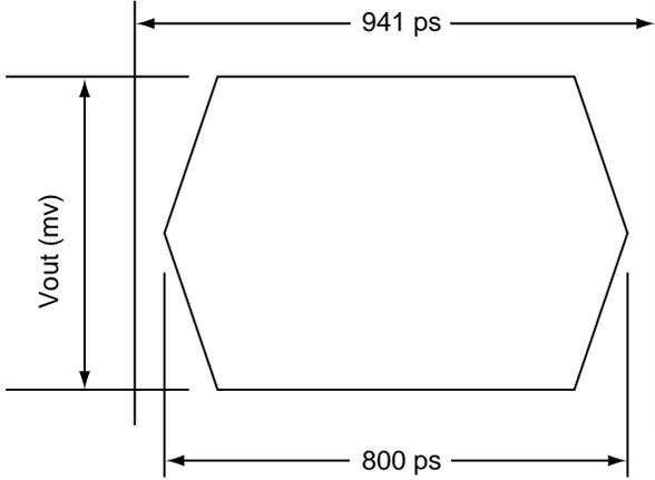
Figure 17. Transmit eye diagram
