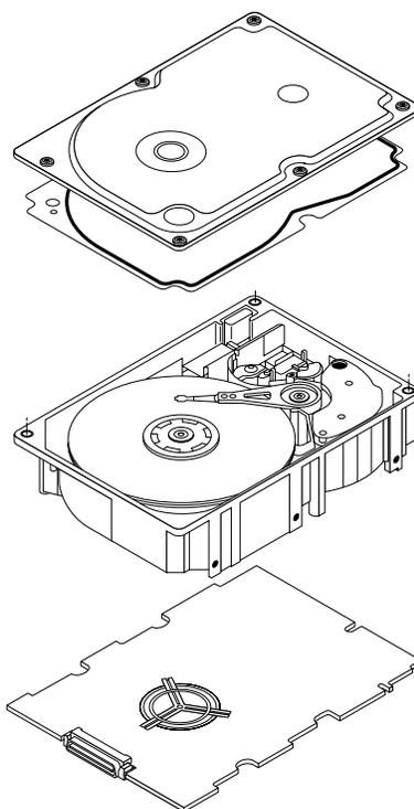
**Figure 2. Barracuda 36FC disc drive**
