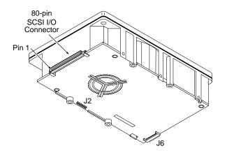
Figure 17. ST1181677LC/LCV drive physical interface (80-pin J1 SCSI I/O connector)
