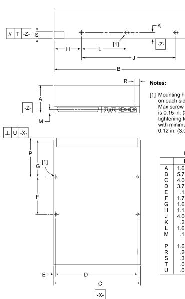
Mounting holes are 6-32 UNC 2B, three on each side and four on the bottom. Max screw penetration into side of drive is 0.15 in. (3.81 mm). Max screw tightening torque is 6.0 in-lb (3.32 nm) with minimum full thread engagement of 0.12 in. (3.05 mm).
