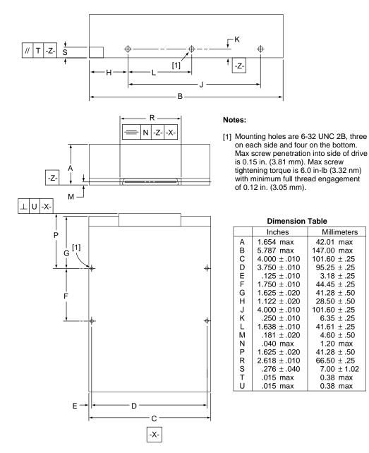
Figure 11. ST1181677LC/LCV mounting configuration dimensions
