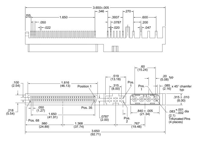
Figure 19. Nonshielded 68 pin SCSI device connector used on LW/LWV drives
