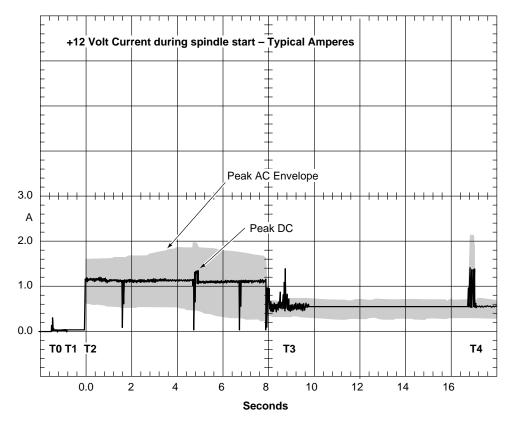
Figure 3. Typical Barracuda 180 family drive +12 V current profile
