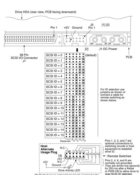
[4] Dashed area is optional host circuitry (external to the drive) connected to host supplied optional usage plug.
