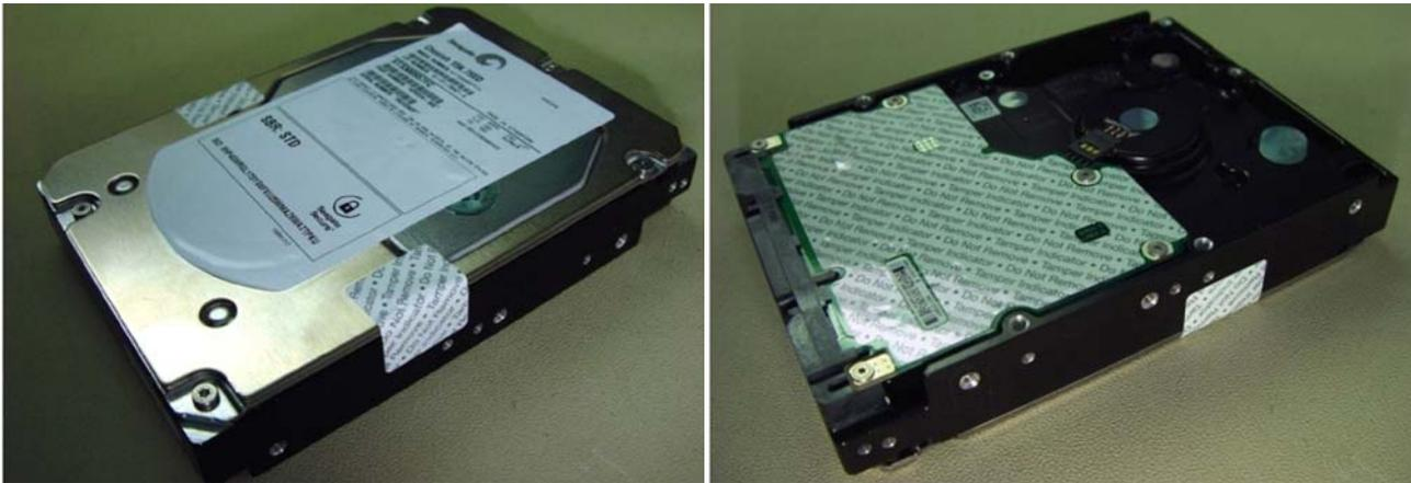
Figure 14. Example of FIPS tamper evidence labels.
