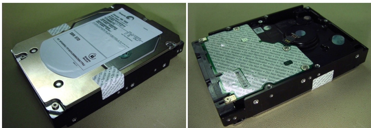
Figure 12. Example of FIPS tamper evidence labels/seals.
