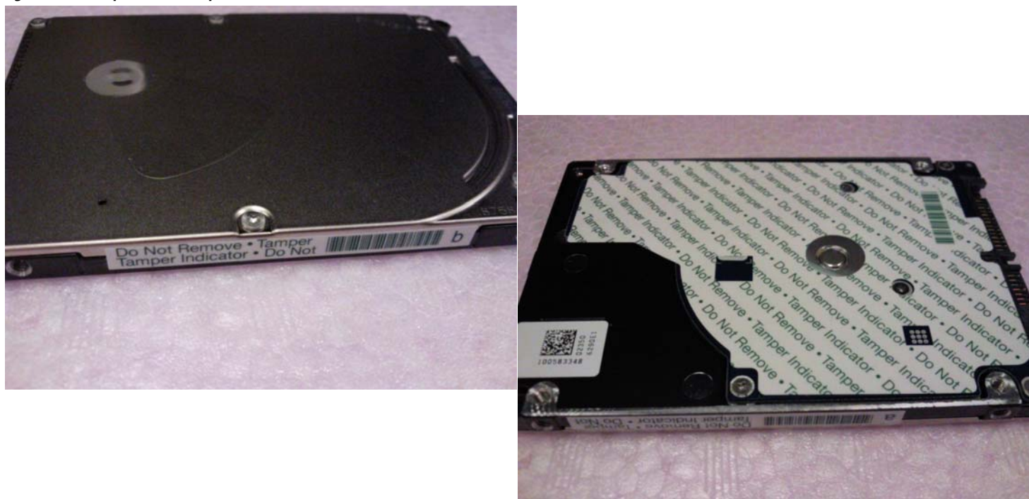
Figure 6 Example of FIPS tamper evidence labels.
