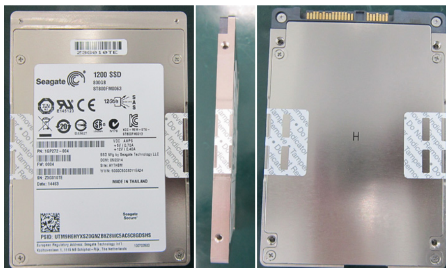
Figure 21. Example of FIPS tamper evidence labels.
