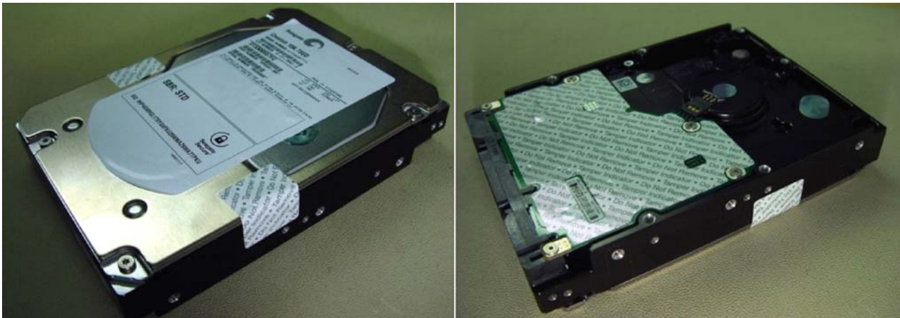
Figure 8. Example of FIPS tamper evidence labels.
