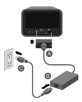
Use only the power supply provided with your device. Power supplies from other Seagate and third-party devices can damage Lyve Mobile Array.
