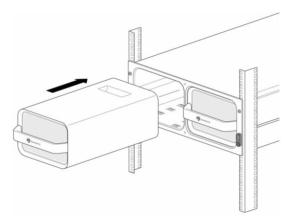
Slide device in until it's fully inserted and firmly connected to Rackmount Receiver's data and power.
