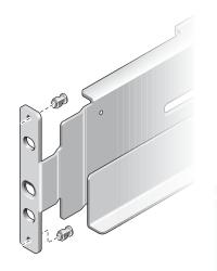
Hanger fasteners (pins) may be pre-installed
