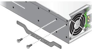
Code A — P/N:01-00000142 2U24 chassis Installed side brackets are shown below in rear panel corner details for 2U12 (left) and 2U24 (right) enclosures.
