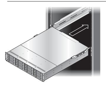
2. Using a total of four  $#10-32 \times 3/4$  truss Phillips or appropriate metric (5 or 6 mm) panhead screws (two per ear), secure the mounting ears on the front of the enclosure to the rack face.
