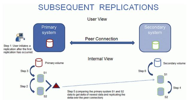
Figure 2 Replication process for replications subsequent to the initial replication.
