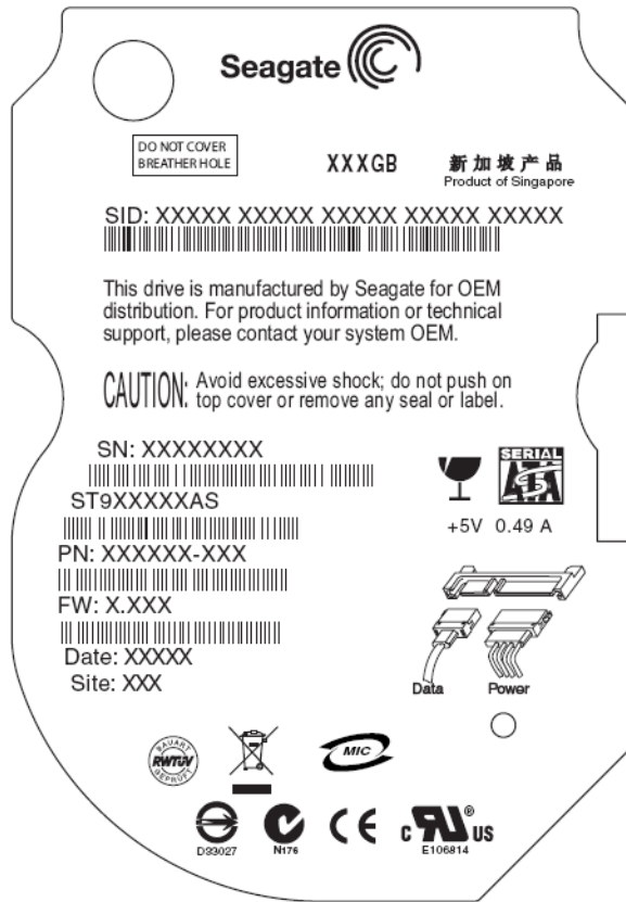
Figure 5. Momentum 7200 FDE.2 SATA drive label example
