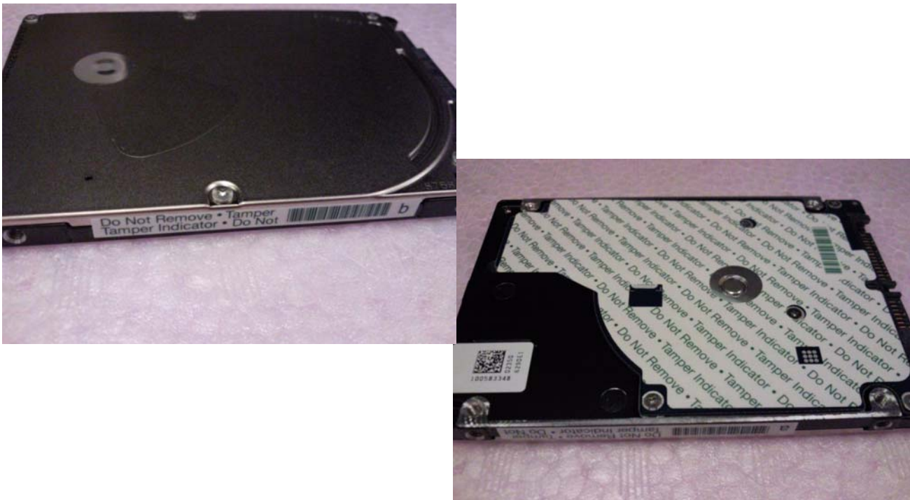
Figure 6. Example of FIPS tamper evidence labels.
