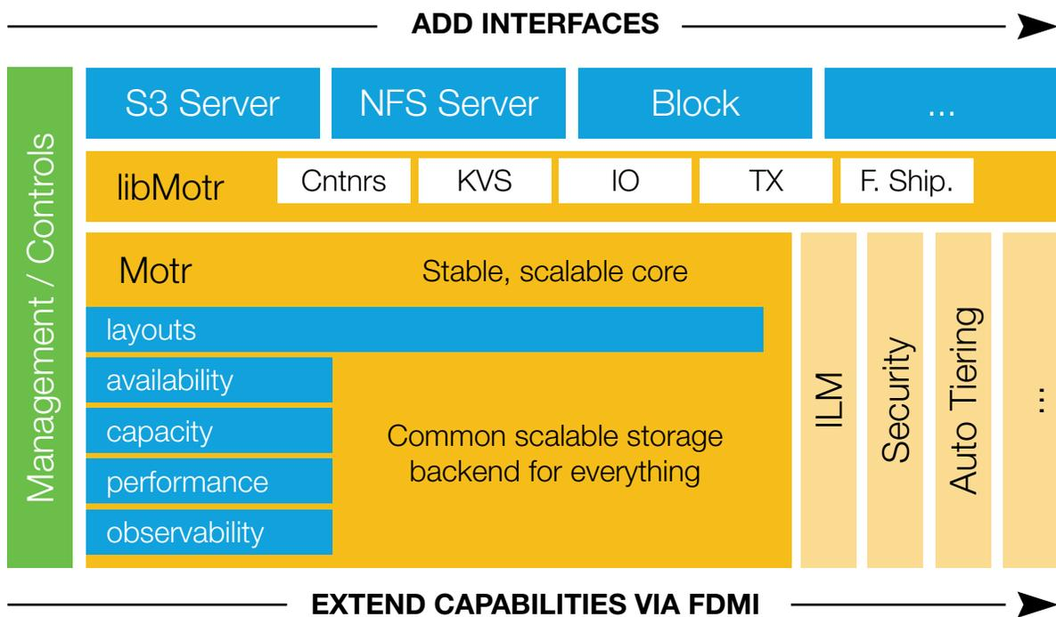
At the core of CORTX is the Motr module, which provides data and metadata storage. Motr uses an internal, RAM-based KVS to store object metadata—i.e., data layouts, access control information, security features, etc.—in a compact,
