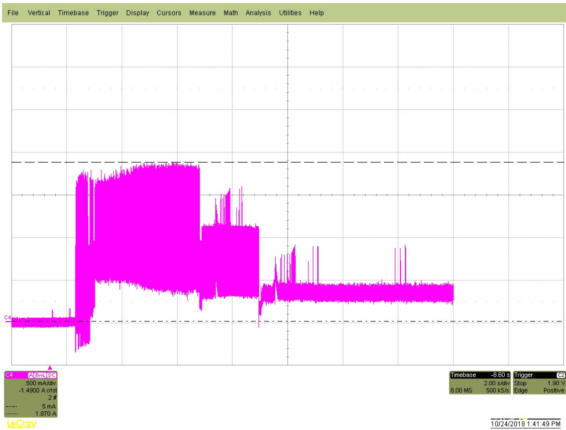
Figure 3. 2TB Typical 12V startup and operation current profile
