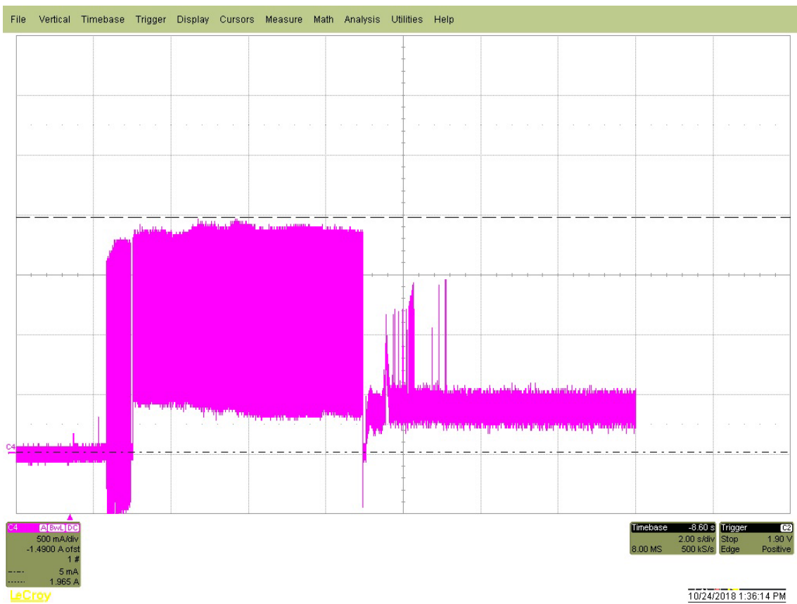
Figure 2. 4TB Typical 12V startup and operation current profile
