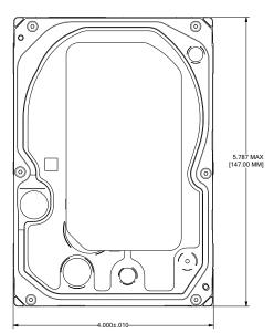
Figure 4. Mounting configuration dimensions 4-disk models
