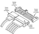
For installations which require cables, users can connect the drive as illustrated in Figure 2.
