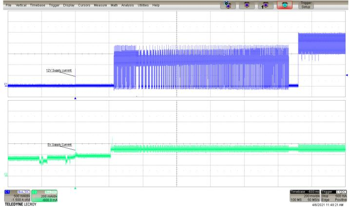
Figure 1. 10TB Typical startup and operation current profile
