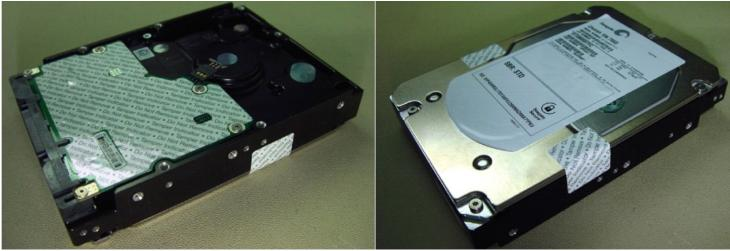
Figure 6. Example of FIPS tamper evidence labels.
