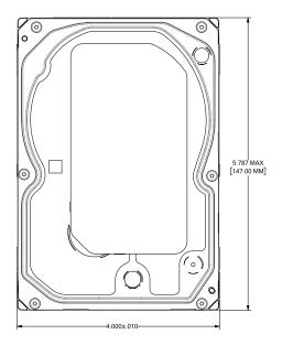
Figure 5. Mounting configuration dimensions 3-disk models
