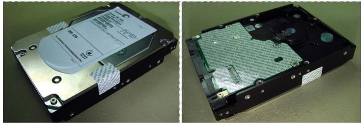
Figure 5. Example of FIPS tamper evidence labels.
