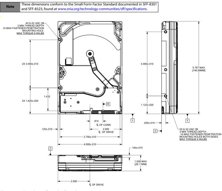
Figure 4. Mounting configuration dimensions
