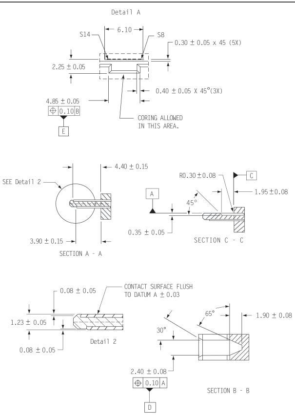
Figure 10. SAS device plug dimensions (detail)
