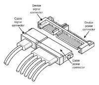
Each cable is keyed to ensure correct orientation. IronWolf drives support latching SATA connectors.
