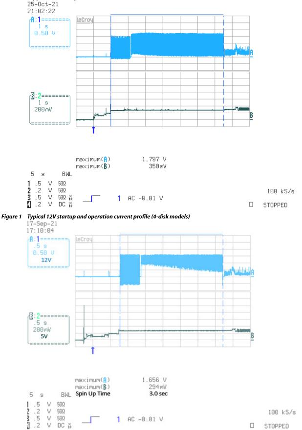
Figure 2 Typical 12V startup and operation current profile (1 and 2-disk models)
