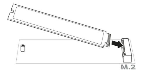
8. Hold down M.2 SSD while you fasten the mounting screw. Make sure the SSD is secured in place.
