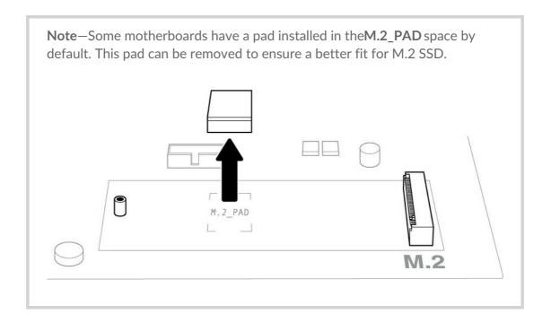
7. Check to make sure that the notch on M.2 SSD is correctly aligned with the divider in the slot. Gently push M.2 SSD into the slot until it's firmly seated.
