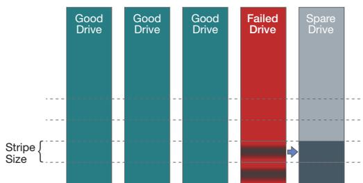
4. Third stripe encounters error from failed drive so data is recovered using good drives.
