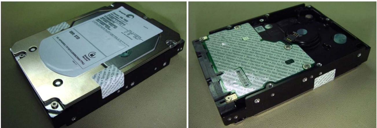
Figure 10. Example of FIPS tamper evidence labels.
