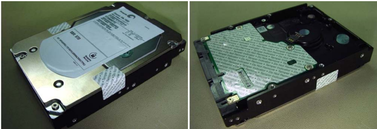
Figure 10. Example of FIPS tamper evidence labels.
