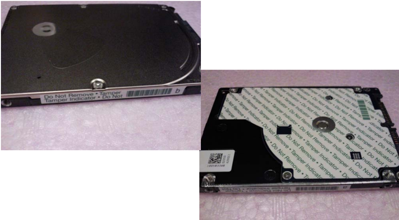
Figure 6. Example of FIPS tamper evidence labels.
