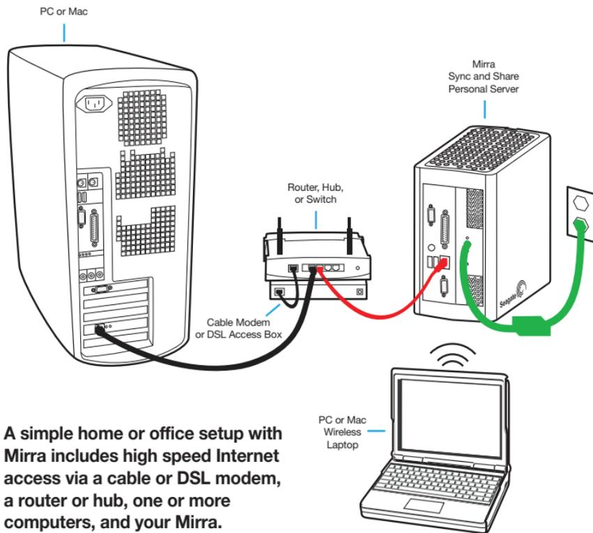
**A simple home or office setup with Mirra includes high speed Internet access via a cable or DSL modem, a router or hub, one or more computers, and your Mirra.**
