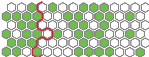
In order to increase areal density, we must shrink the volume of the grains on the media (represented by “V” in the formula below). When we do this, the grains become thermally unstable unless we also increase the anisotropy of the media (represented by “K”). Remember, anisotropy is the degree of difficulty required to change the magnetic orientation of grains on the media.
