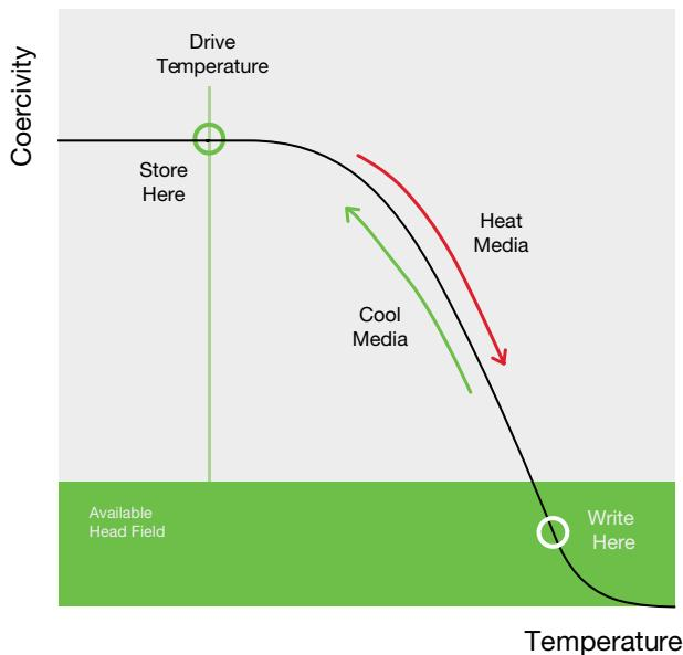
We write the media when it is hot, and store it when it is cold (see illustration left). The entire process—heating, writing, and cooling—takes less than 1 nanosecond.
