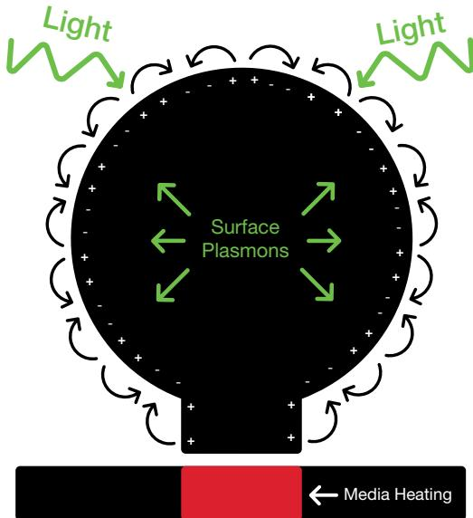
The Seagate plasmonic NFT works on the same principle. Our plasmonic NFT consists of a disk and a peg. Light is absorbed by the disk and turned into a surface plasmon. This surface plasmon travels along the outside edge of the disk and down the peg, heating that precise point on the media. The width of the peg is the width of the hot spot on the media. This is much smaller than the diffraction limit—and that's how we beat the diffraction limit.
