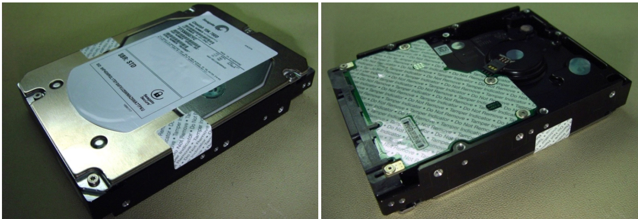
Figure 5. Example of FIPS tamper evidence labels.
