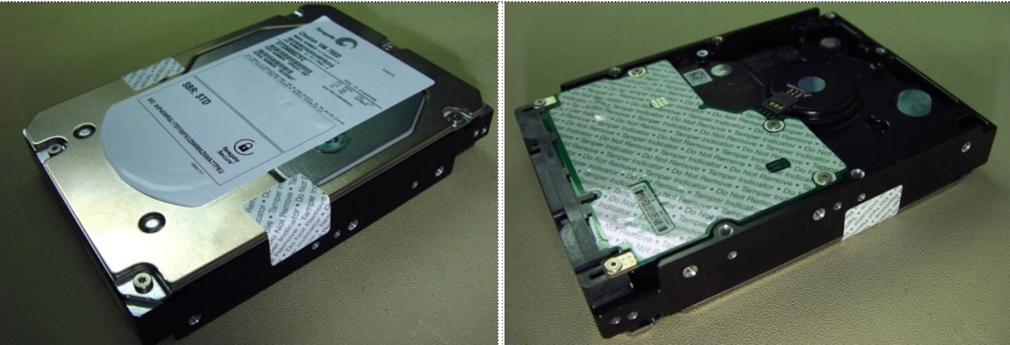
Figure 11. Example of FIPS tamper evidence labels.
