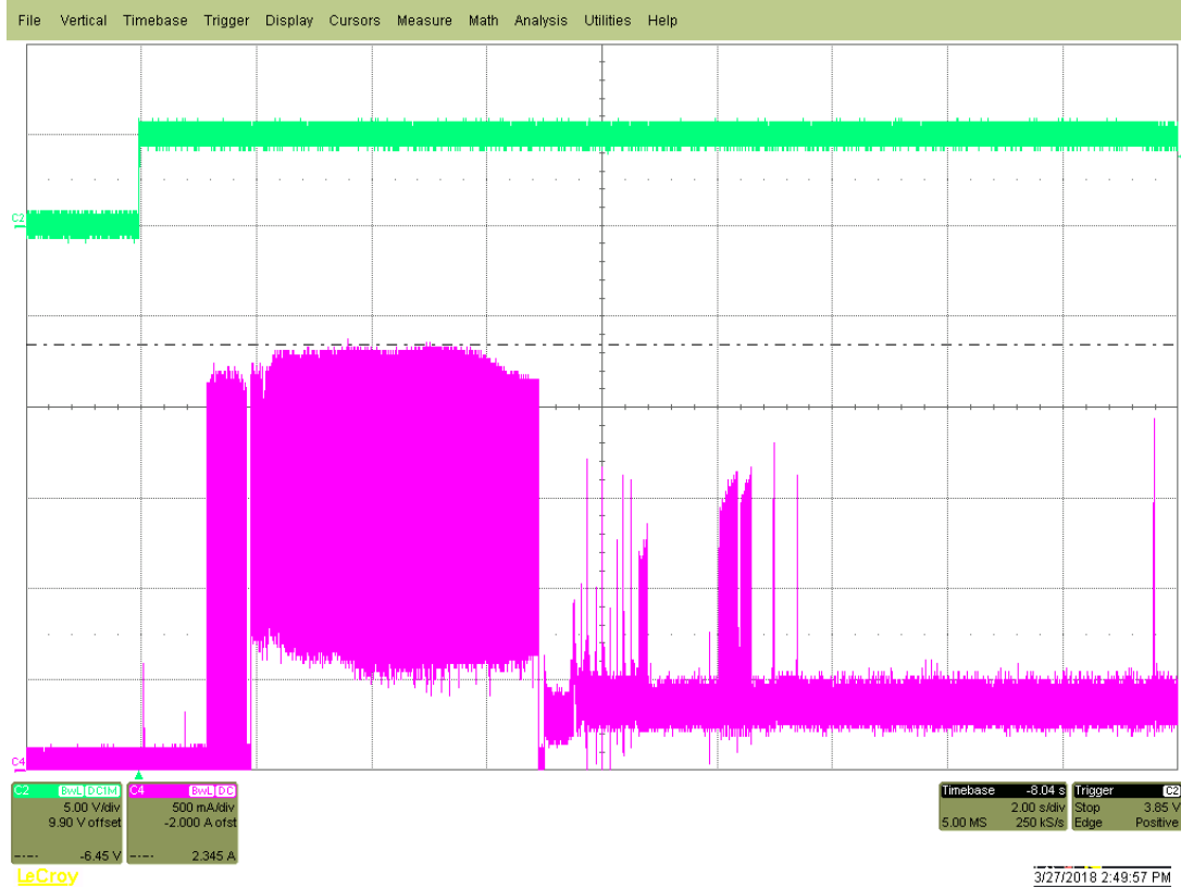
Figure 1. Typical 5V and 12V startup and operation current profiles
