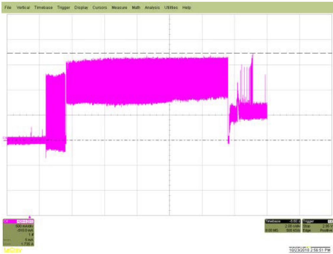
Figure 1. 8TB & 6TB Typical 12V startup and operation current profile
