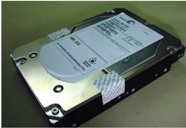
Figure 14. Example of FIPS tamper evidence labels.
