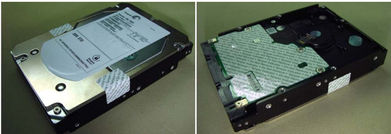
Figure 16. Example of FIPS tamper evidence labels.
