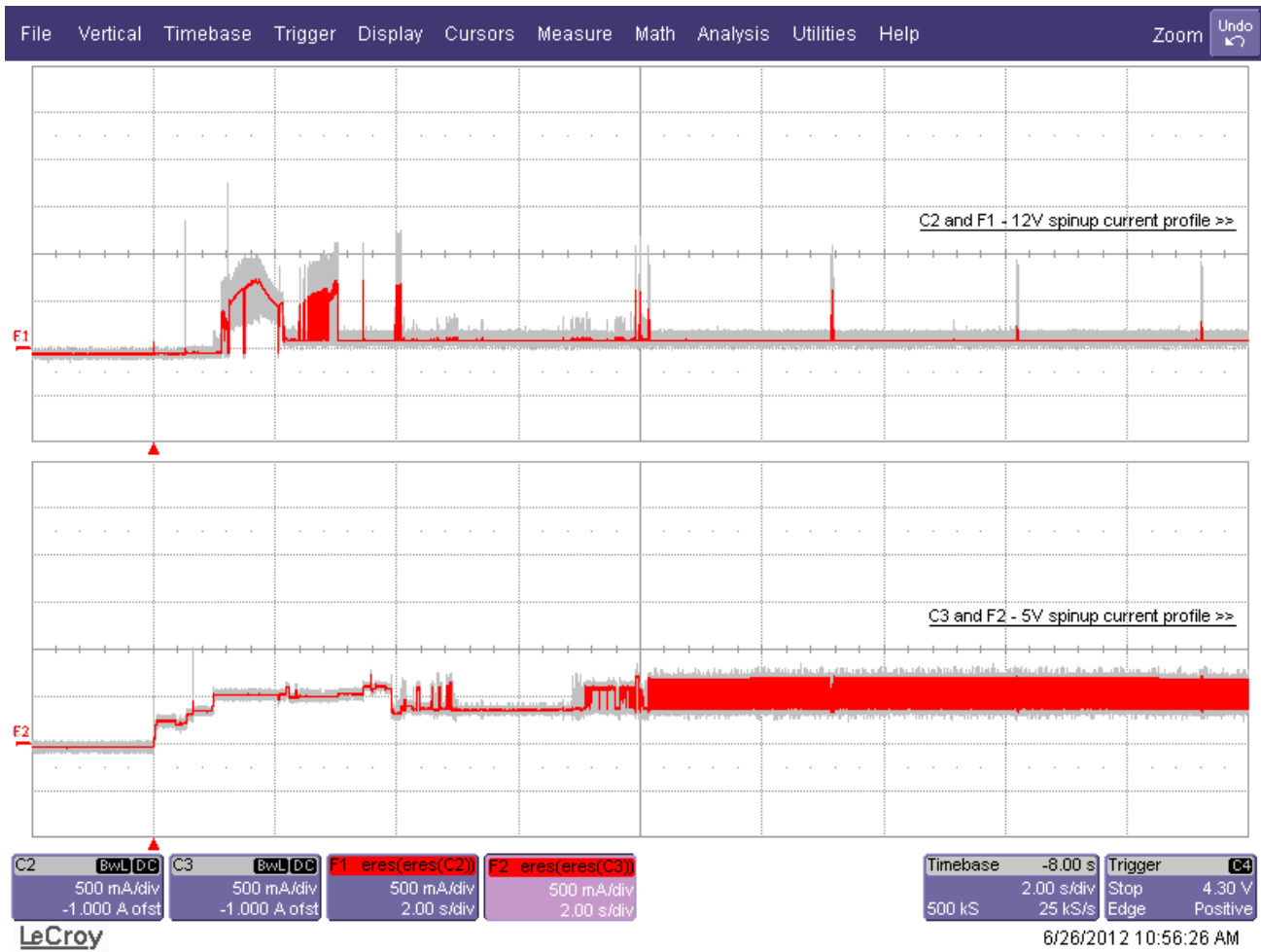
Figure 4. Current profiles for 300GB models
