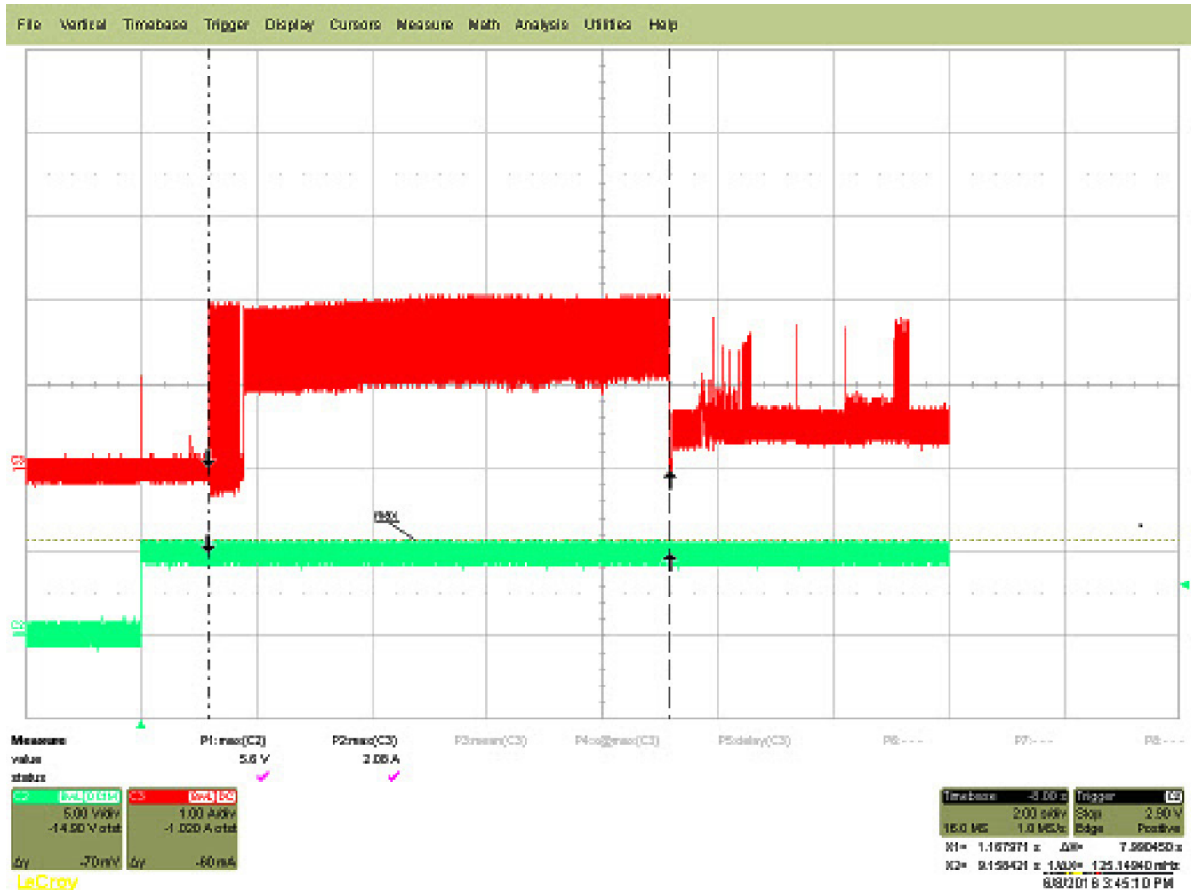
Figure 1 6TB Typical 5V and 12V startup and operation current profiles
