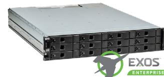
*Ideal primary storage for small and mid-size studios. Excellent balance of price, performance, and capacity. Capable of up to 7GB/s aggregate reads when combined with additional 2u12 expansion chassis.*
