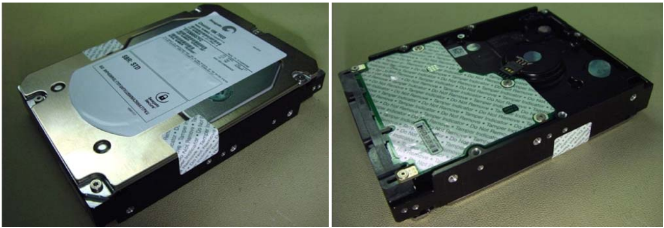
Figure 10. Example of FIPS tamper evidence labels. Note. Image is for reference only, may not represent actual drive.
